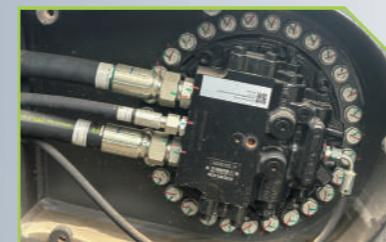
Adopting a large diameter main valve, optimizing the valve core structure, reducing the friction between hydraulic oil and plumbing, and reducing oil duct pressure loss was reduced by more than 20%.
