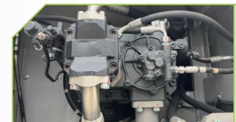
Adopting a large diameter main valve, optimizing the valve spool structure, reducing the friction between hydraulic oil and plumbing, and reducing oil duct pressure loss was reduced by more than 20%.
