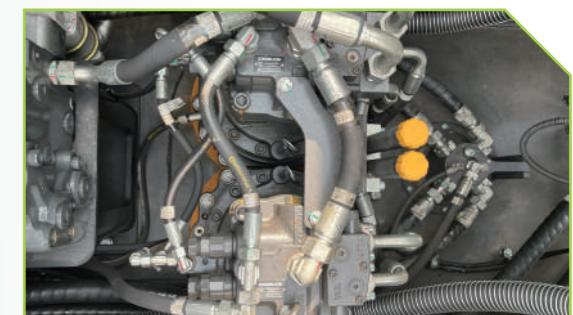
Large displacement dual swing motor, mature technology, large swing torque, fast start, and fast swing speed.
