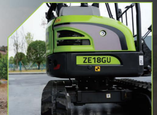
One of ZE18GU's highlights is zero tail swing, its radius of swing will not exceed the width of the track in the full expanded state. This design means that it can work in narrow spaces and on busy roads, not limited by space.
