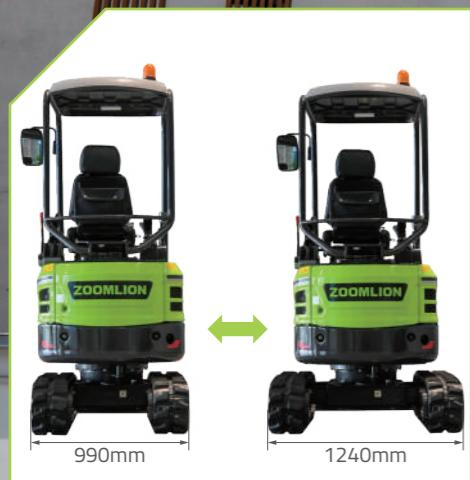
Retractable track, so that the width of the machine is adjustable from 990 mm to 1240mm. In a narrow working space, the track shrinks so that the width of the whole machine becomes smaller, and the passability is better.
