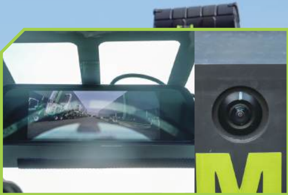
Optional reversing camera Its large display at the front of the cab and the high-definition camera at the rear ensure a complete view of the machine's rear door.
